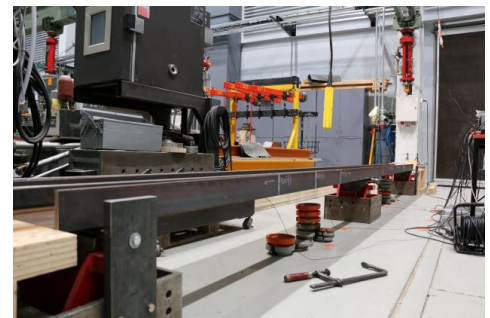
(b) Continuously supported beam (CSB)
