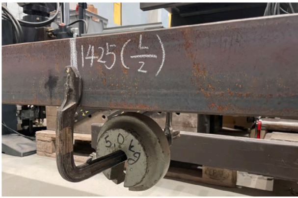
Fig. 7. Bridge with additional mass (5 kg).
