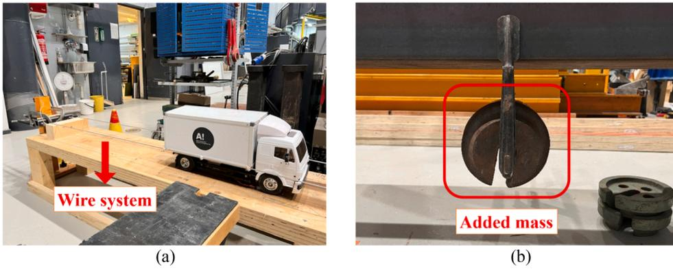
Fig. 17. Setup for the lab test: (a) wire system, (b) added mass at the mid-span.
